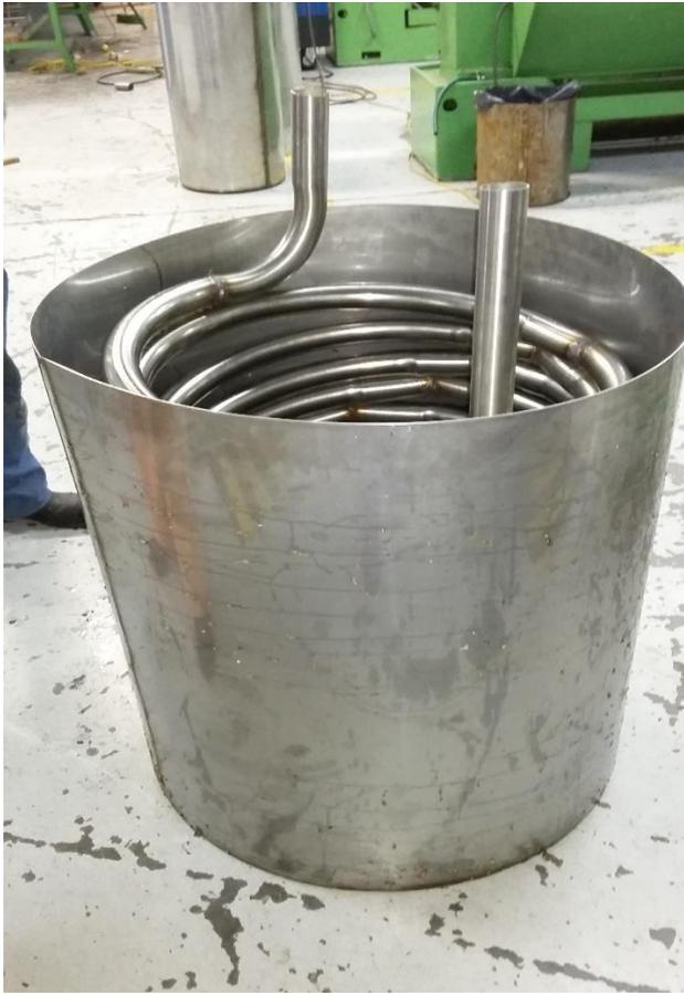
**Figura 4.5 - Reactor tubular**
